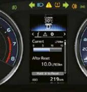
Optitron Meter Combination with Colour Multi-Information Display
